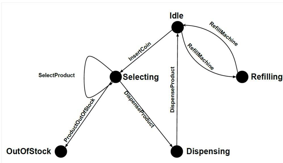
**Figure 4.** LTS illustration of a simple vending machine
